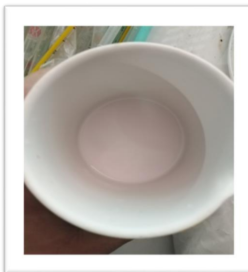
Figure 2.12: Faint pink color of milk at the end of titration
