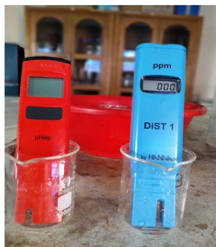
TDS and pH determination using TDS meter and pH meter
