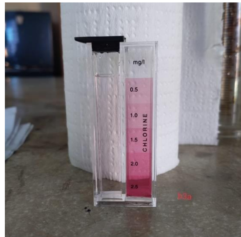
Color comparing to measure the Free Chlorine in ppm.
