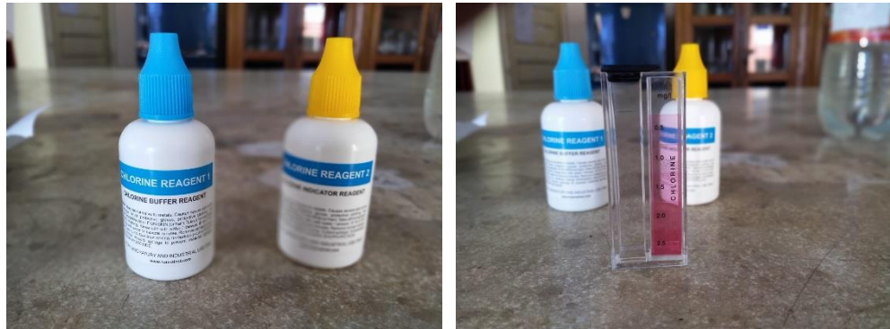
Reagent Kit and Testing tube for color comparison used in free Chlorine determination
