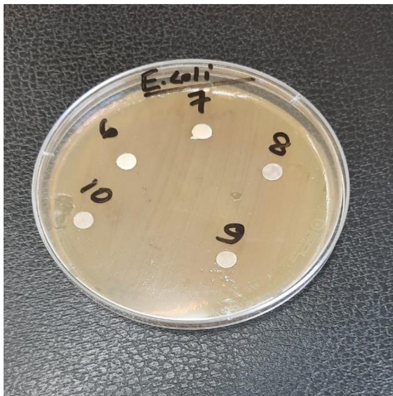
Figure 4. 2: Petri dish with samples 6, 7, 8, 9, 10 with no inhibition zone
