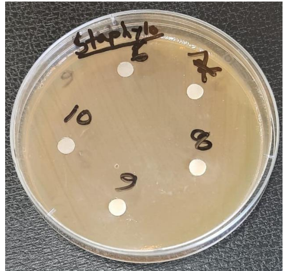
Figure 4. 3: Petri dish with samples 6, 7, 8, 9, 10 with no inhibition zone
