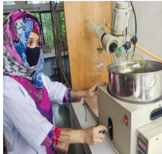
Extraction by rotary evaporator
