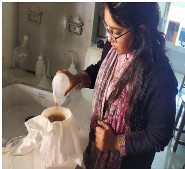
Figure 4. Filtration of the mixture for CF analysis
