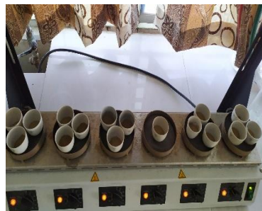
Figure 8. Sample being burnt for ash estimation
