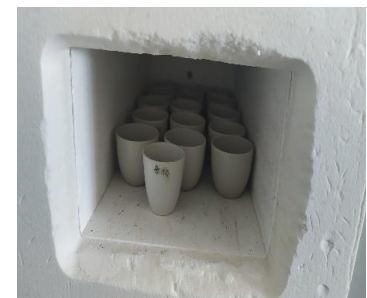
Figure 9. Samples given in the muffle furnace for ash estimation
