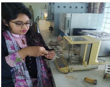
Figure 7. Sample weighing for EE estimation
