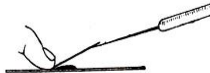
Fig. 42. METHOD OF PUTTING THE COVERSLIP
