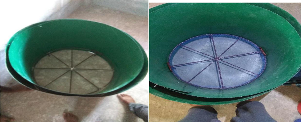
Fig 3: circle of two plain sheet( body of incubator)
