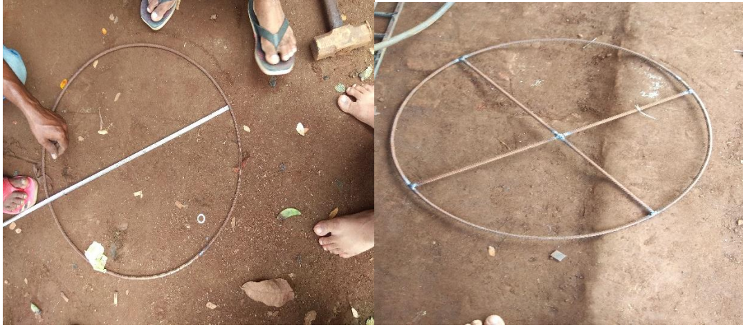
Fig 1: making circular ring by bending the rod
