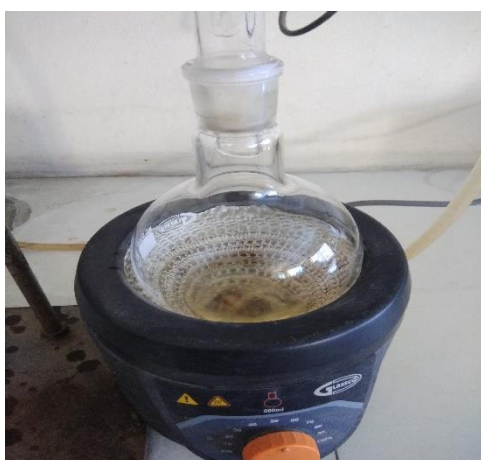
Reflux condenser (Saponification determination)
