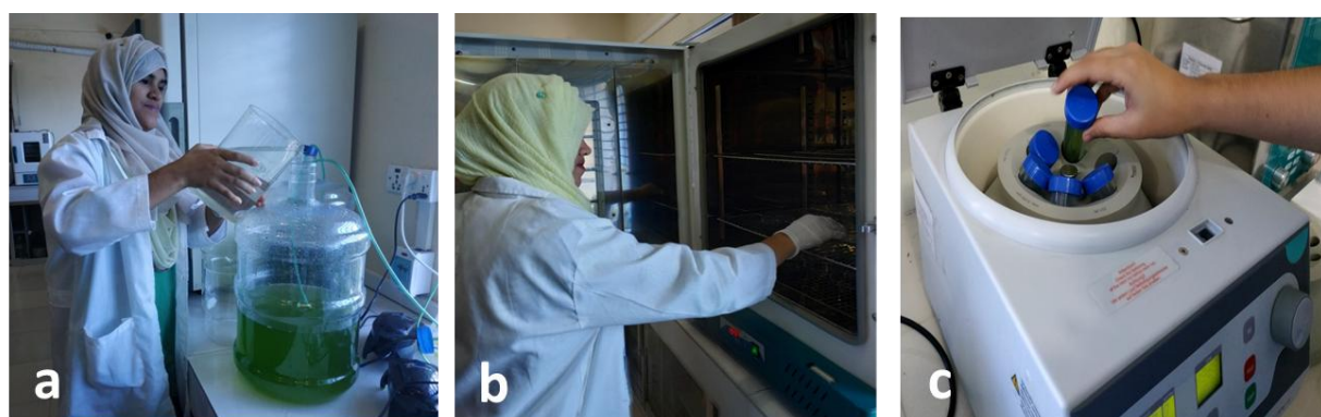
Figure 2 Laboratory activities regarding culture of microalgae. a) mass-culture of microalgae and addition of culture media, b) drying microalgae extracts in a hot air Oven at 60°C for 12h, c) harvesting microalgae by centrifugation.
