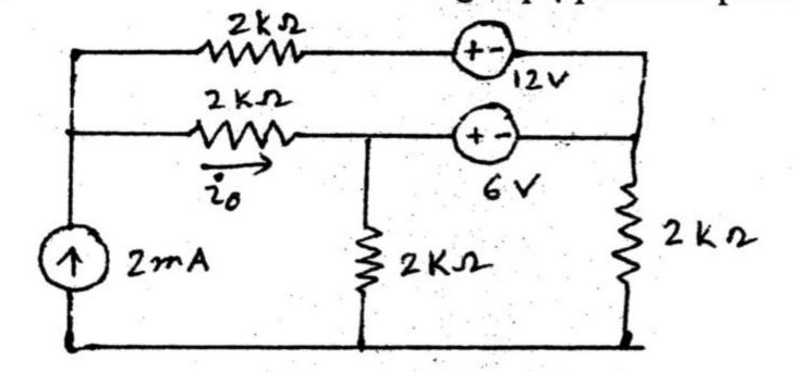
b) Find the Thevenin and Norton equivalent circuits at the terminals a-b for the circuit below:
