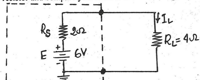
Reduce the network of figure below to a single current source and calculate the current through R<sub>L</sub>.
