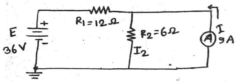
b) Using superposition theorem, determine the current through the  $12\Omega$  resistor.
