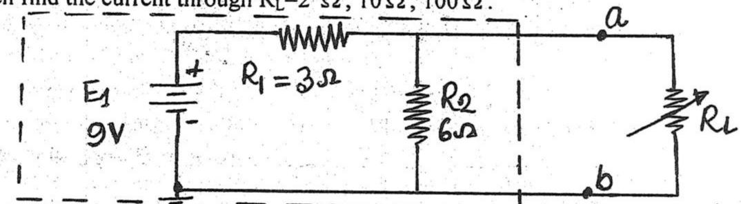
b) Maximum power transfer occurs when the load voltage and current are one-half their maximum possible values,- Prove.
