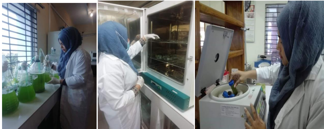
Figure 2 Laboratory activities regarding culture of microalgae. (Left) mass-culture of microalgae and addition of culture media, (middle) drying microalgae extracts in a hot air oven at 60°C for 12h, (right) harvesting microalgae by centrifugation.
