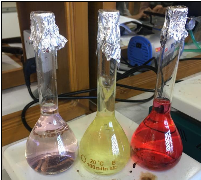
Plate 3: Preparation of main minerals stock solution (100 g/L NaNO 3 ), trace metals solution, vitamin solutions
