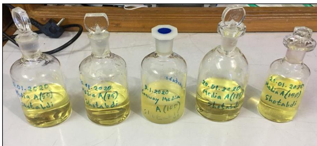
Plate 5: Main minerals stock solution with 50 g/L, 75 g/L, 100 g/L (Control), 125 g/L and 150 g/L concentration of Sodium nitrate ( \text{NaNO}_3 )
