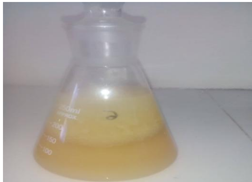
Fig A3: Extraction of pectin from malta peel using citric acid and nitric acid
