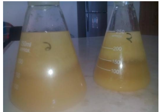
Fig A3: Extraction of pectin from malta peel using citric acid and nitric acid
