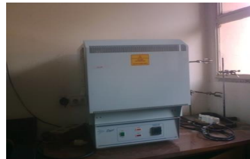
Figure D5: Furnace used to ash the sample.
