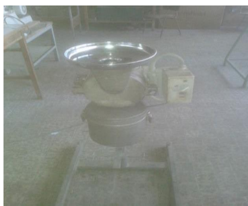
Figure: 3.1. Cross beater mill with hopper
