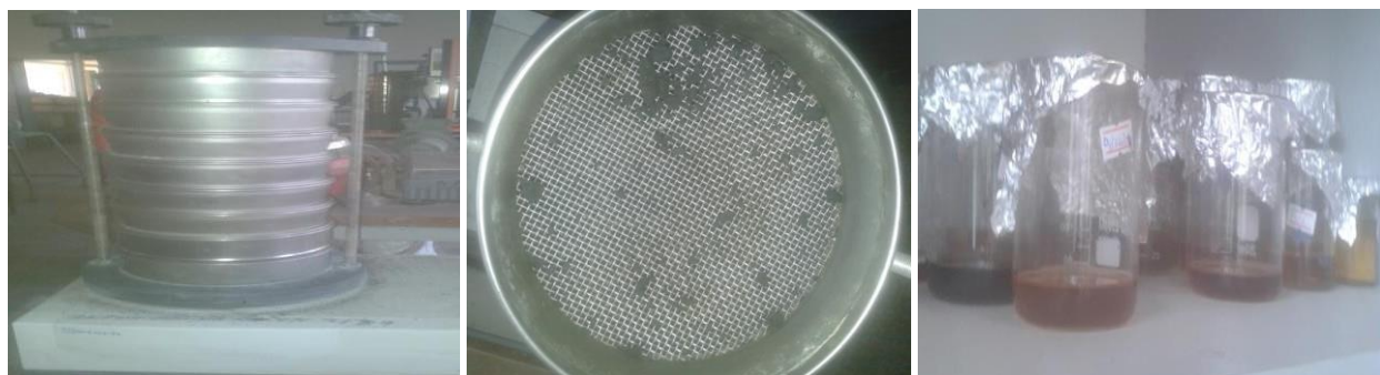
Figure D12: Sieve shaker, Sieve in top view, Samples of black cumin extracted essential oil respectively.
