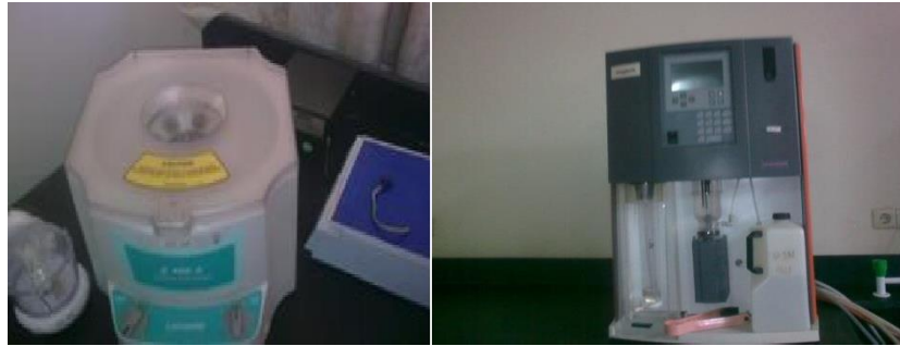
Figure D9: Centrifuge used to separate components of a complex mixture Figure D10: Kjeldahl analyzer unit which is used for protein analysis that is distillation and titration.
