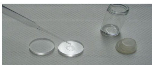
Figure D17: Fourier Transform Infrared Sample holder of liquid and equipment
