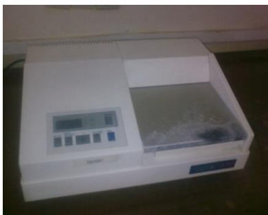
Figure D6: UV-visible Spectroscopy used to measure absorbance of Ur analyst of interest,
