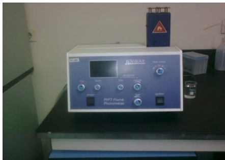
Figure D4: Flame photo meter used to detect Na & K
