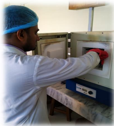
Fig B5: Determination of ash content
