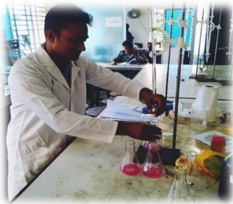
Fig B3: Determination of titrable acidity
