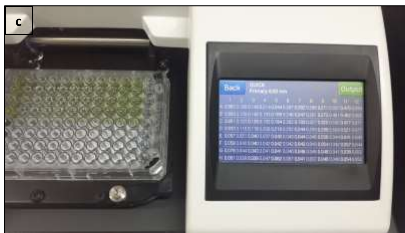
Appendix T: (a) Cyanobacterial extracts in microtiter plate (96-well), Minimum inhibitory concentration determination of Oscillatoria Strain 2 M2 (25) (b) and Strain 4 Fw2 (c) in ELISA machine
