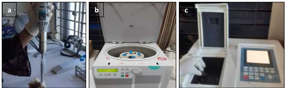
Appendix I: Chlorophyll content estimation (a) Homogenizing the sample, (b) Centrifugation of the sample (c) Spectrophotometric analysis
