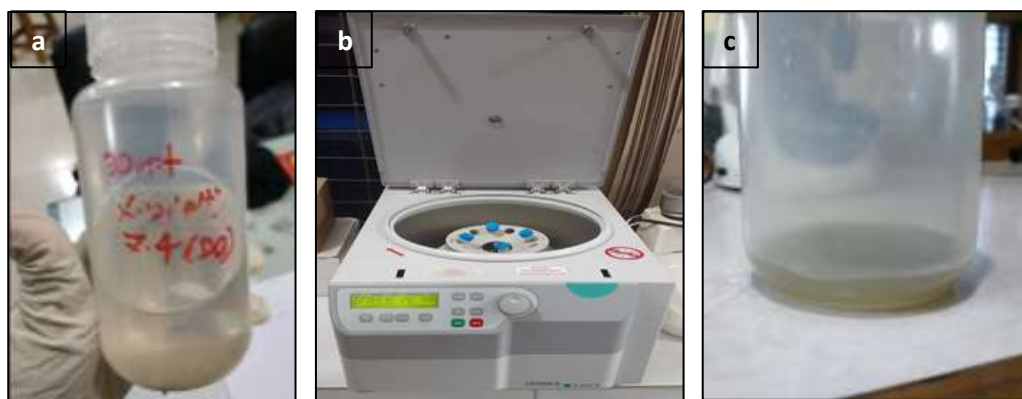
Appendix C: (a) Water sample from the sampling sites, (b) Concentration of sample, (c) Concentrated sample
