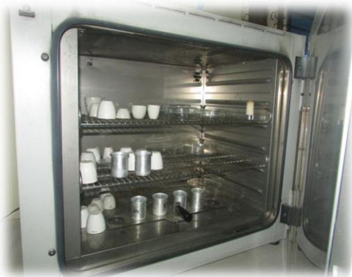
Figure 2: Estimation of DM by Using Hot air oven & Desiccators
