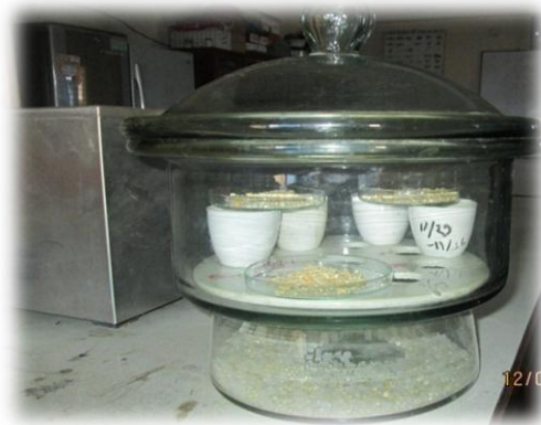
Figure 2: Estimation of DM by Using Hot air oven & Desiccators
