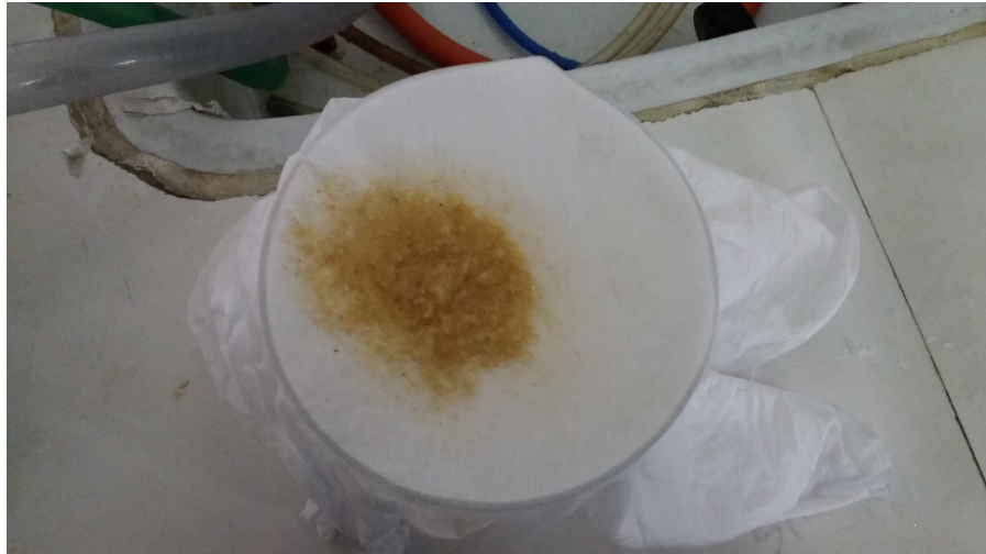
Figure A25: Filtration to separate water insoluble fiber
