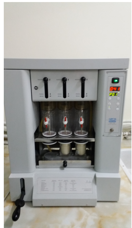
Figure A31: Sample in Soxhlet apparatus for fat determination
