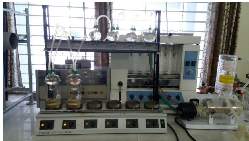
Figure A24: Boiling with alkali and acid
