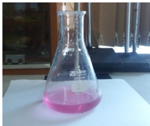
Plate 6: Solution after titration for CO 2
