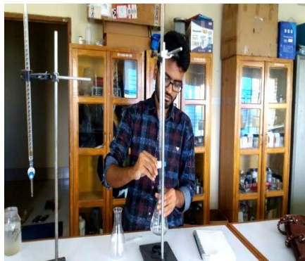
Plate 3: Titrating the sample
