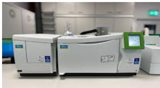
Figure 3.4: Gas chromatography for fatty acid determination
