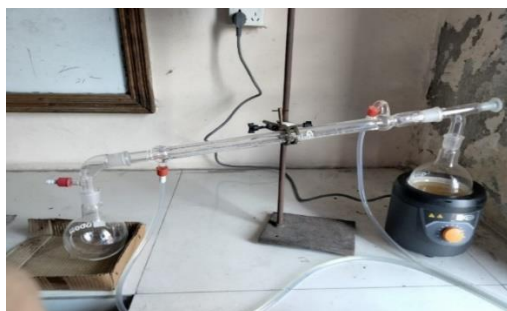
Figure 3.14: Liebig Condenser with sample
