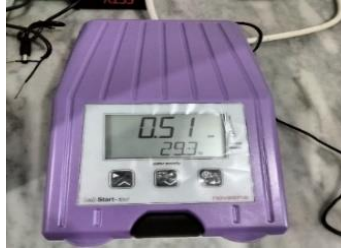
Figure 3.3: Novasina Digital Water activity meter (Model: Lab start, swift and touch)
