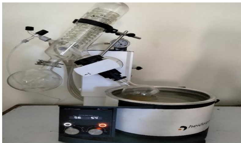
Figure 3.11: Rotary evaporator (category: Heidolph) with sample
