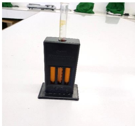
Figure 3.18: Measurement of haemoglobin by Sahli's hemoglobinometer.
