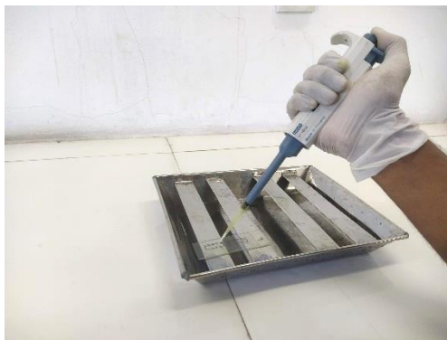
Figure 3.14: Milk sample was placed on slide to make smear
