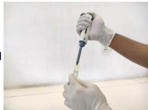
Figure 3.15: 0.01ml of milk sample was taken using micropipette
