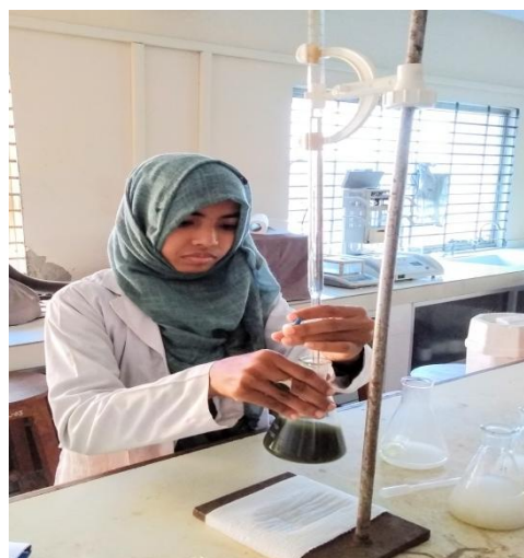
Titration with 0.1N \text{Na}_2\text{S}_2\text{O}_3 solution
