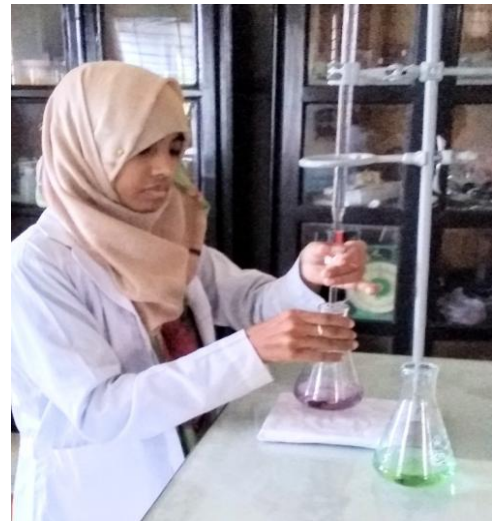
Titration with 0.1N HCl
