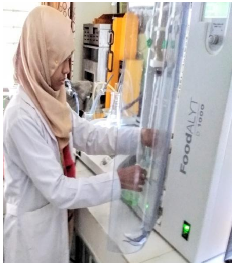
Collecting distillate from distillation flask
