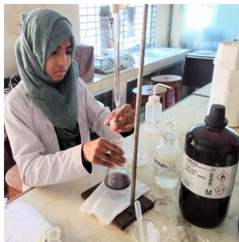
Titration with unknown \text{Na}_2\text{S}_2\text{O}_3 solution
