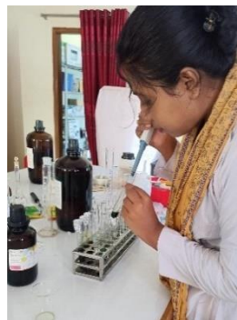
Sample Preparation for UV visible Spectrophotometer
