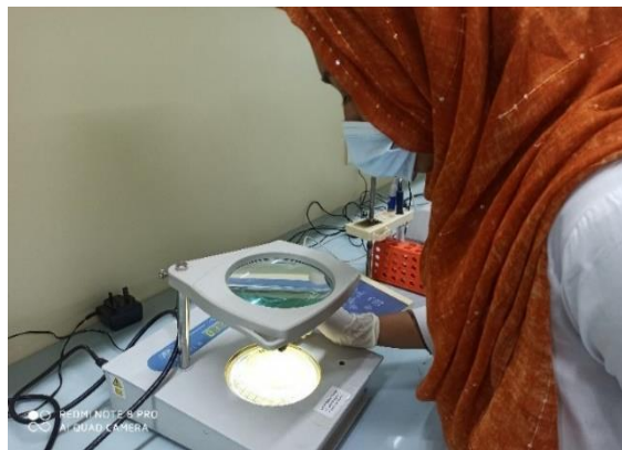
Figure 7 : Counting of bacteria in a colony counter
