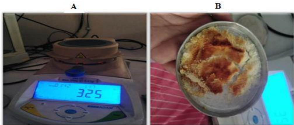
(A) Moisture analyzer machine, (B) After burning of the powdered milk in the analyzer
