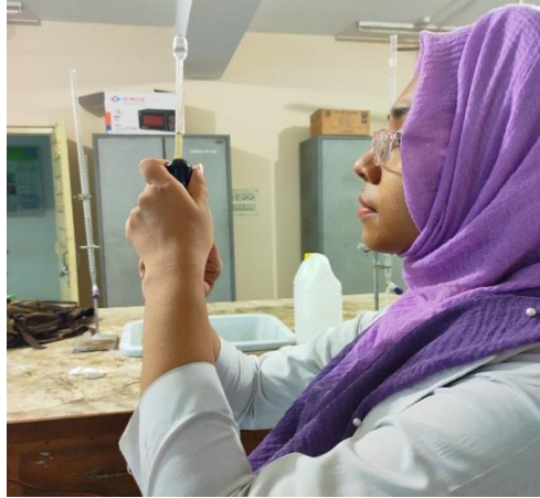
Figure 3: Reading of fat recorded from butyrometer at vertical position
