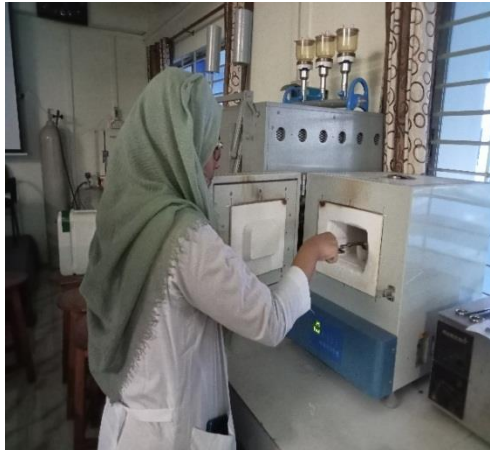
Figure 6 : Placed sample in a muffle furnace
