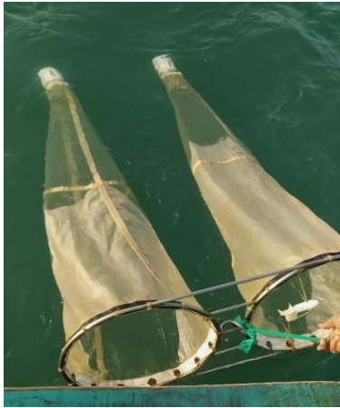
Plate 1. Sampling by bongo net
