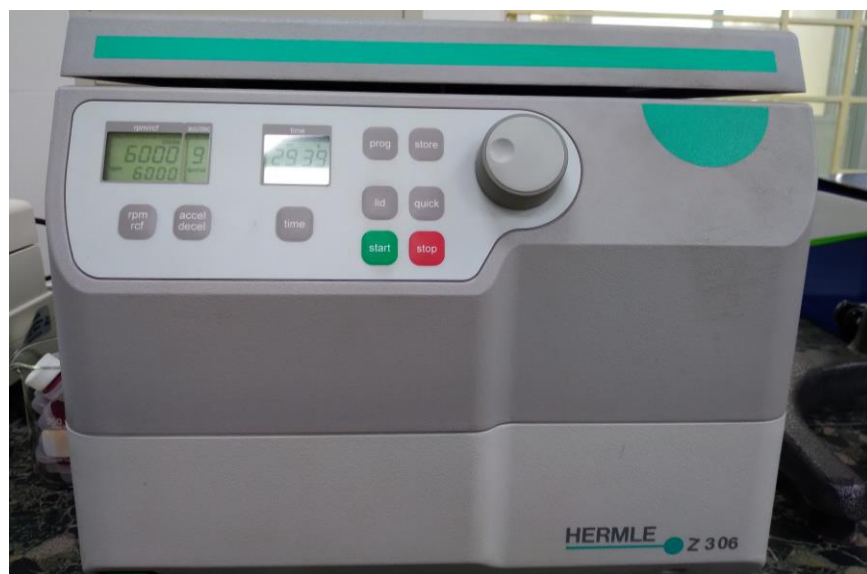
Figure B03: Centrifuge device used for layer separation
