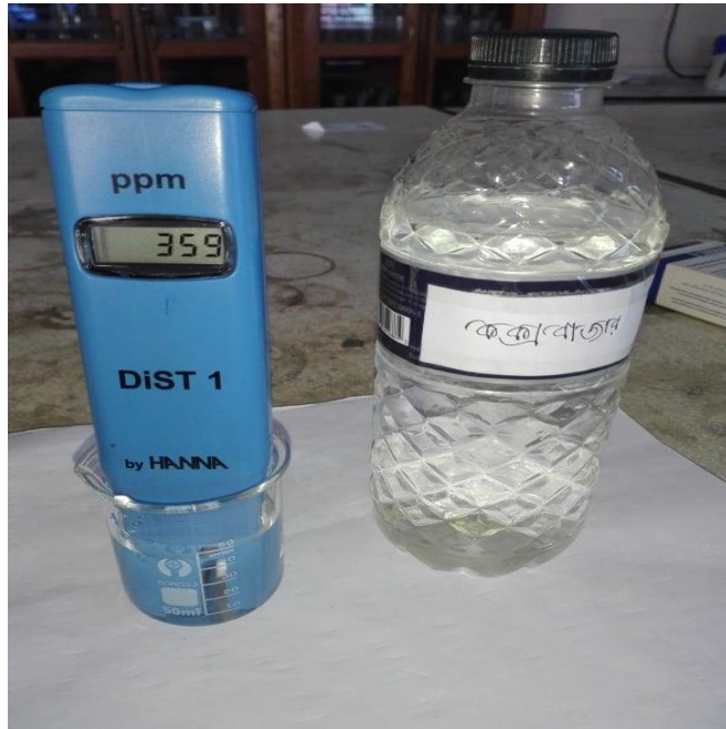
TDS measurement of Rain Water Sample
