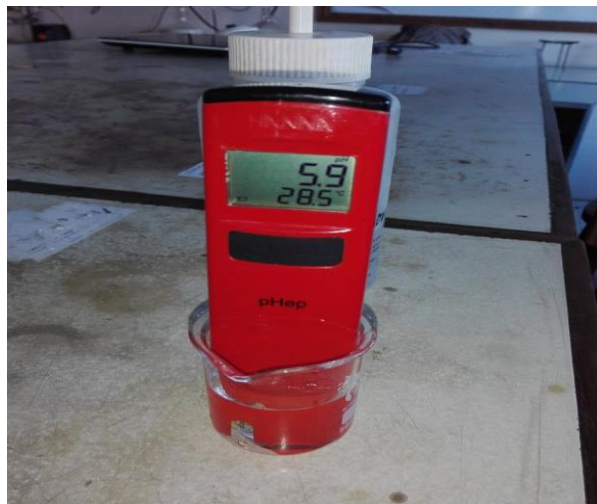
P H measurement of Rain Water Sample
