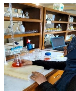
Plate 9: Titrating for Alkalinity
