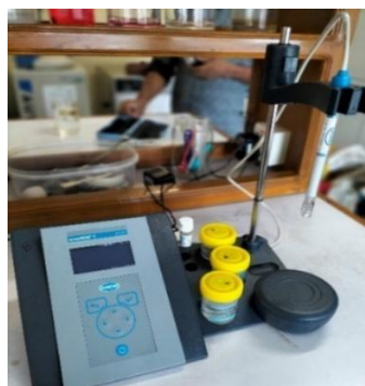
Plate 2: TDS meter (HACH sensION+EC71)
