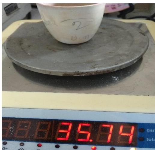
**Figure 3.4: Moisture Analysis using hot air oven.**
