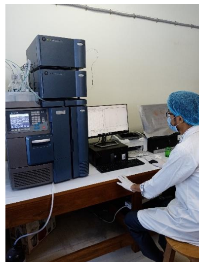
Determining Amino Acid Profile using HPLC
