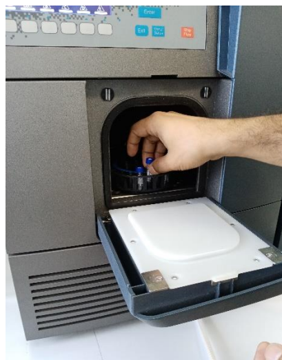
Determining Amino Acid Profile using HPLC
