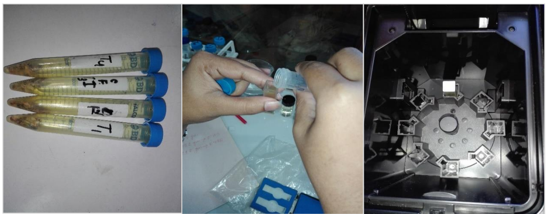
(a) (b) (c) Plate-11: (a) Extracted sample after freezing (b) taking sample for carotenoid content analysis (c) putting sample in spectrophotometer at 470 nm wave length
