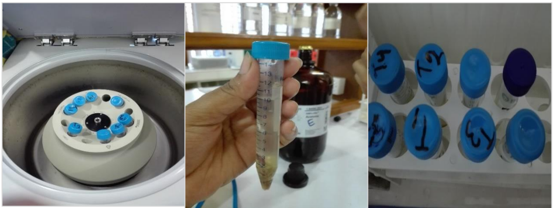
(a) (b) (c) Plate-10: (a) Sample putting into centrifuge machine at 5000 rpm for 5 min (b) taking out from centrifuge machine (c) putting these sample in freeze for 72 hrs
