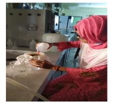
Figure 5. Acid boiling for CF estimation
