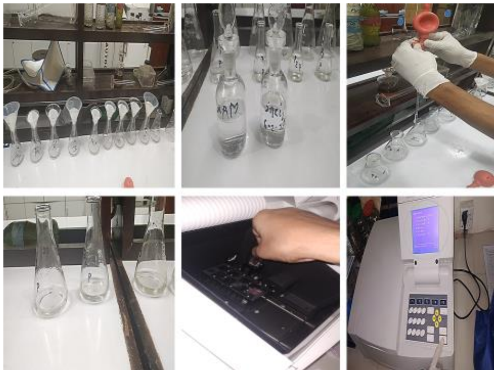
Figure 14: Determination of phosphate; a) filtration of sample, b) Required chemicals, c) Adding chemicals, d) Reaction, e) Insertion of vial, f) Photometric measurement
