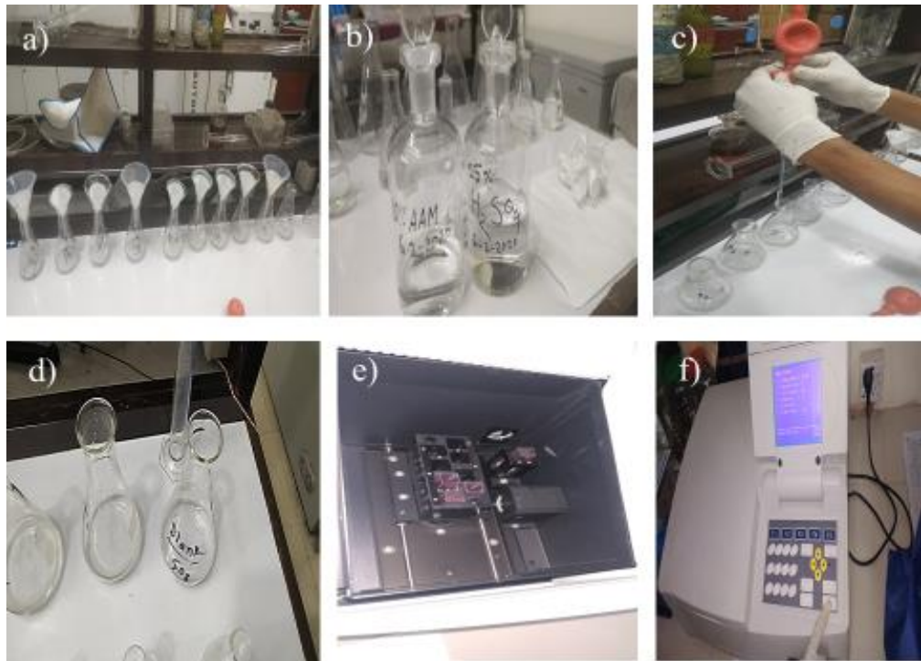
Figure 15: Determination of silicate; a) Filtration on sample, b) Required chemicals, d) Adding chemicals, d) Ongoing reaction, e) Insertion of vials, f) Photometric measurement
