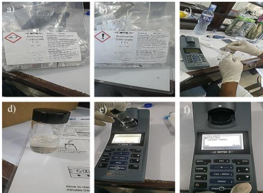
Figure 12: Ammonia determination of sample; a) and b) Required reagents c) Adding reagents, d) Ongoing reaction, e) Inseting vial, f) Ammonia analysis
