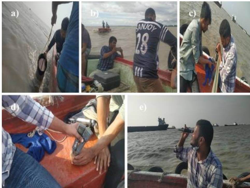
Figure 17: Field work: a) and b) Phytoplankton net towing, c) Insertion plankton sample in plastic bottle, d) pH measurement, e) Salinity measurement
