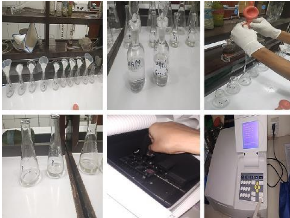
Figure-10 : Determination of phosphate; a) filtration of sample, b) Required chemicals, c) Adding chemicals, d) Reaction, e) Insertion of vial, f) Photometric measurement
