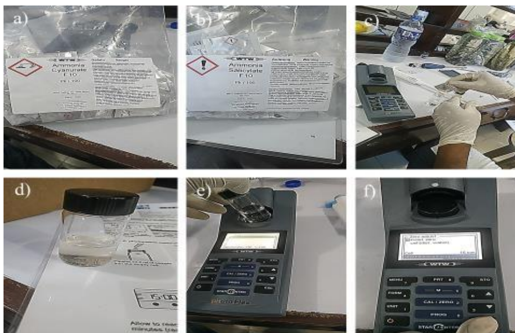
Figure-9 :Ammonia determination of sample; a) and b) Required reagents c) Adding reagents, d) Ongoing reaction, e) Inseting vial, f) Ammonia analysis
