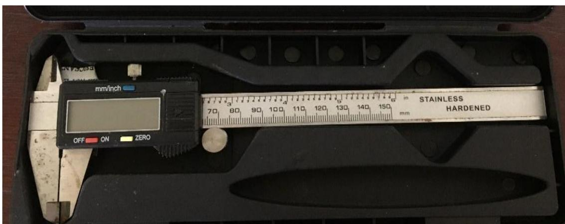
Figure 6 Digital Slide Calipers used to measure length
