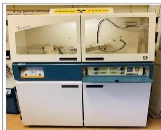
Figure 3.6. X-ray powder diffractometer for \text{CaCO}_3 analysis
