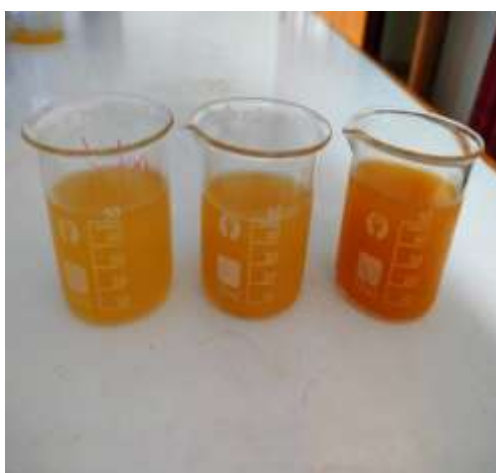
Pineapple juice sample after treatment(thermal, microwave, sonicated respectively)
