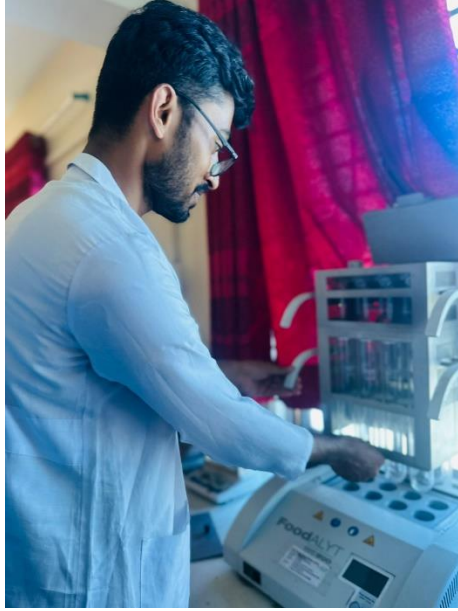
Figure: Protein determination by KJELDAHL method
