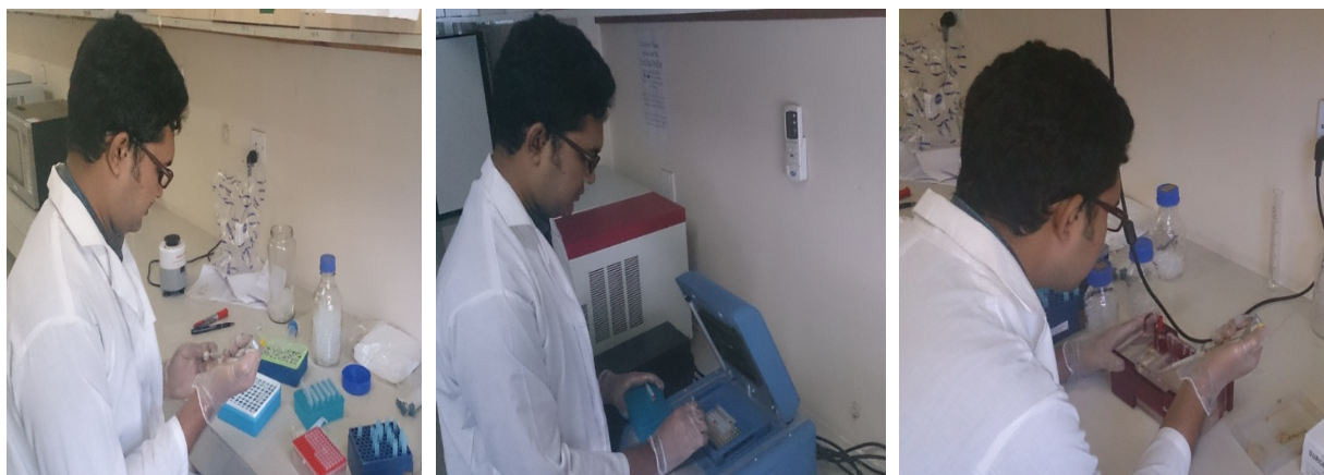
Adding reagents for PCR Placing Samples in PCR machine Filling Gel pores with samples
