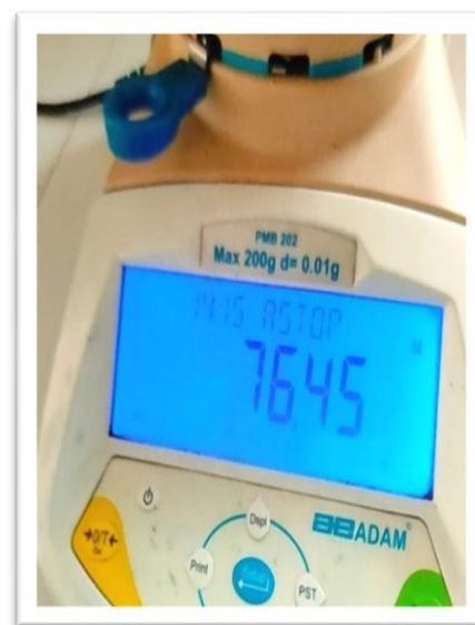
Figure 14: Moisture percentage measured by PMB 202 Analyzer
