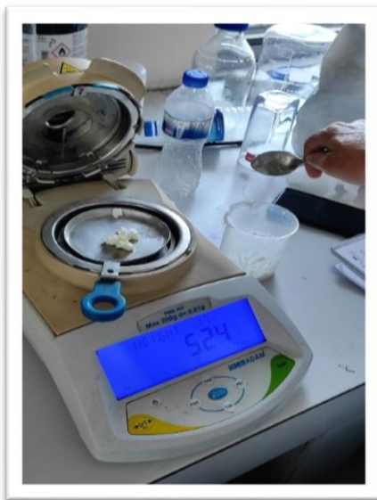
Figure 13: Weighing of dahi by PMB 202 Analyzer
