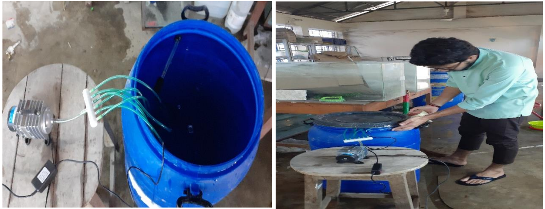
Appendix C: Water purification through continuous aeration and UV radiation
