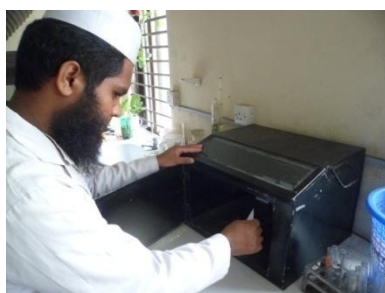
Placing of plate at UV chamber samples
