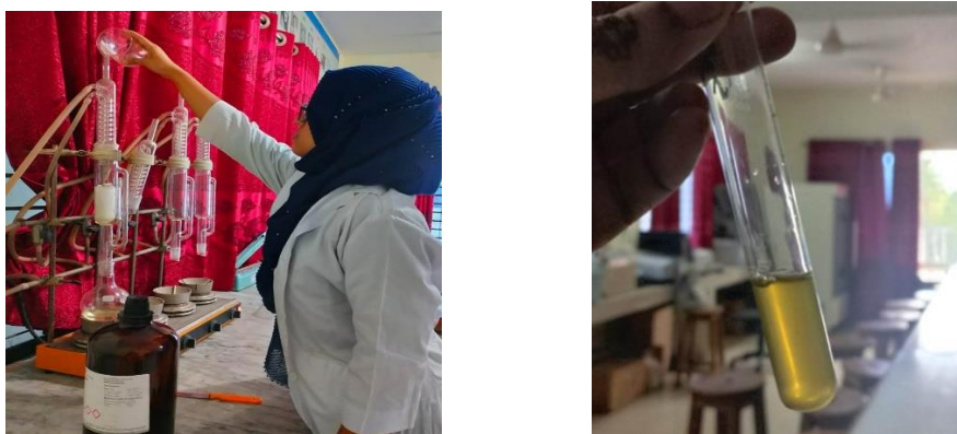
Seed oil preparation by Soxhlet apparatus
