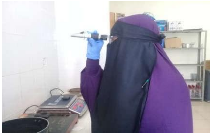
Testing Brix value using refractometer
