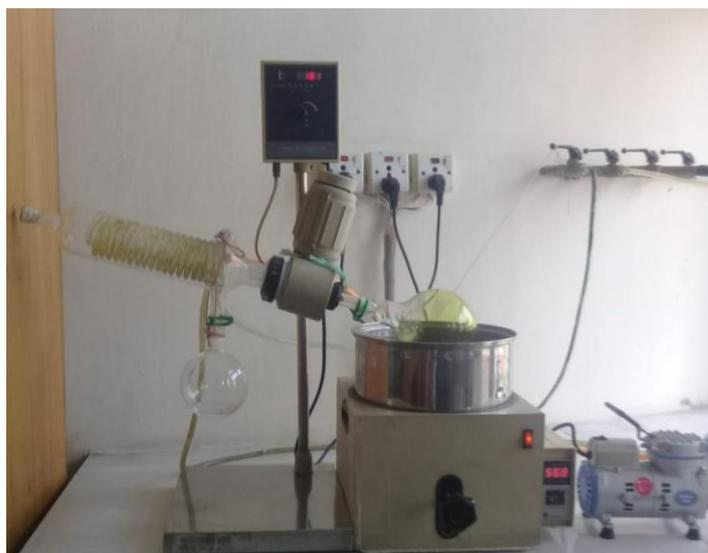
Figure 3.4: Rotary evaporator used for solvent extraction.
