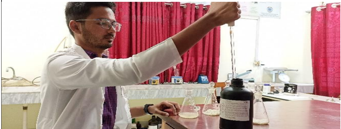
Digestion of samples with 30% 100 ml H_2O_2
